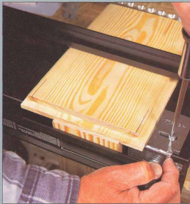
Photo 9 Left-hand edge guide being tightened against the edge of the drawer front
