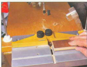
Routing the detail on the drawer front edges
