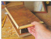
Adding the trim to the cut edges of the veneered ash
