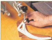
Cutting the internal detail first on the scrollsaw
