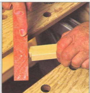
Rounding the tenons with a Permagrit rasp
