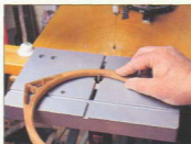
Routing the edge decoration on the Proxxon miniature router table
