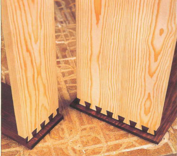
Photo 2 Flush offset and full rebate drawer fronts. The full rebated front is not quite symmetrical
