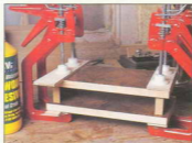
The base unit clamped to set the glue
