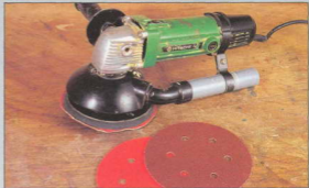
Above Hand-sanding an edge - there are times when machine sanding isn't possible Right A random orbital sander will give very good results
