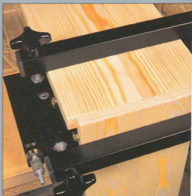
Photo 6 A drawer side clamped vertically against the stop pin. A backing board horizontally behind it prevents breakout
