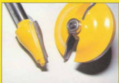
There are two ways to raise a panel, either with a vertical or flat safety pattern cutter
