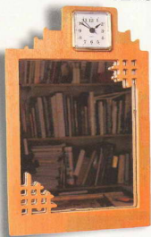
An art deco style mirror frame scrollcut from a 1/2in panel recovered from a piano case
