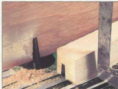
Photo 6 Spline/taper – Note the use of the through fence for edge cut
