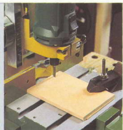
Making the template for frame slotting
