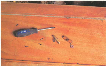
Dismantling an upright piano front panel reveals \frac{1}{4} in thick sheets of mahogany
