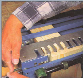
Photo 11 The vertical stop being set to an offset, equal to the width of the rebate plus 12mm. This example results in an offset of 24mm
