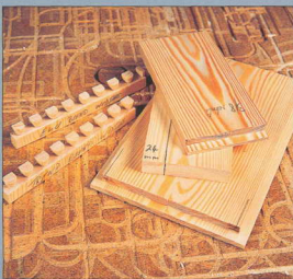
Photo 3 Useful work aids - two board-width pieces, a rebate board, rebated edge-guide gauge and a 24mm offset setting piece
