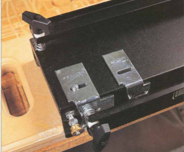
Photo 7 The Trend jig with edge guide No. 2 at left-hand end and normal No. 1 at right-hand end. The left-hand No. 1 is placed on the jig to show the difference in offsets between the two
