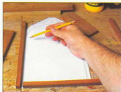
Marking up the frame blanks for cutting
