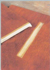
Above The effect of cross-grain scratching has been exaggerated but it shows just how bad it can look
