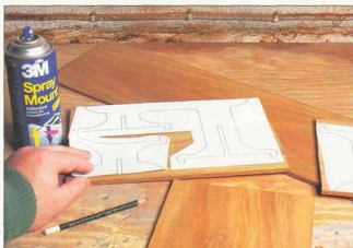
Laying out a set of cutting patterns on a recovered panel. The components will end up as an indoor plant stand
