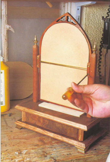
Fitting the mirror in place with the clamping brackets
