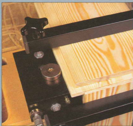
Photo 5 A rebated drawer front set horizontally in the DeWalt jig, with the rebate board clamped vertically to bring the raised portion of the front flush with the front of the jig, and the spacer washer mounted on the stop pin to offset the front
