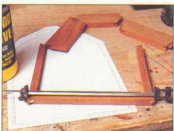
The first two frame joints mitred, biscuited and clamped to set
