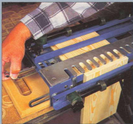
Photo 10 Setting up the Titan jig for the drawer front. The rebated front is flush with front of jig and centred under the template
