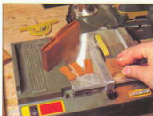
Cutting the jointing 'biscuits' from offcuts of the same wood as used for the frame
