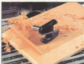
Photo 3 Panel raiser – a clean result
